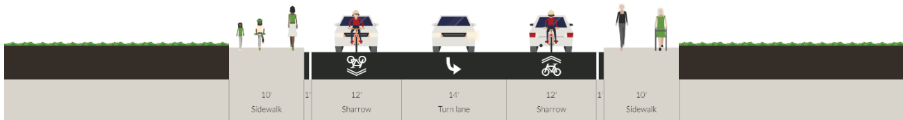
Arterial with Center Turn Lane – Intersection Treatment (60-foot ROW, 40-foot Paved Width)
